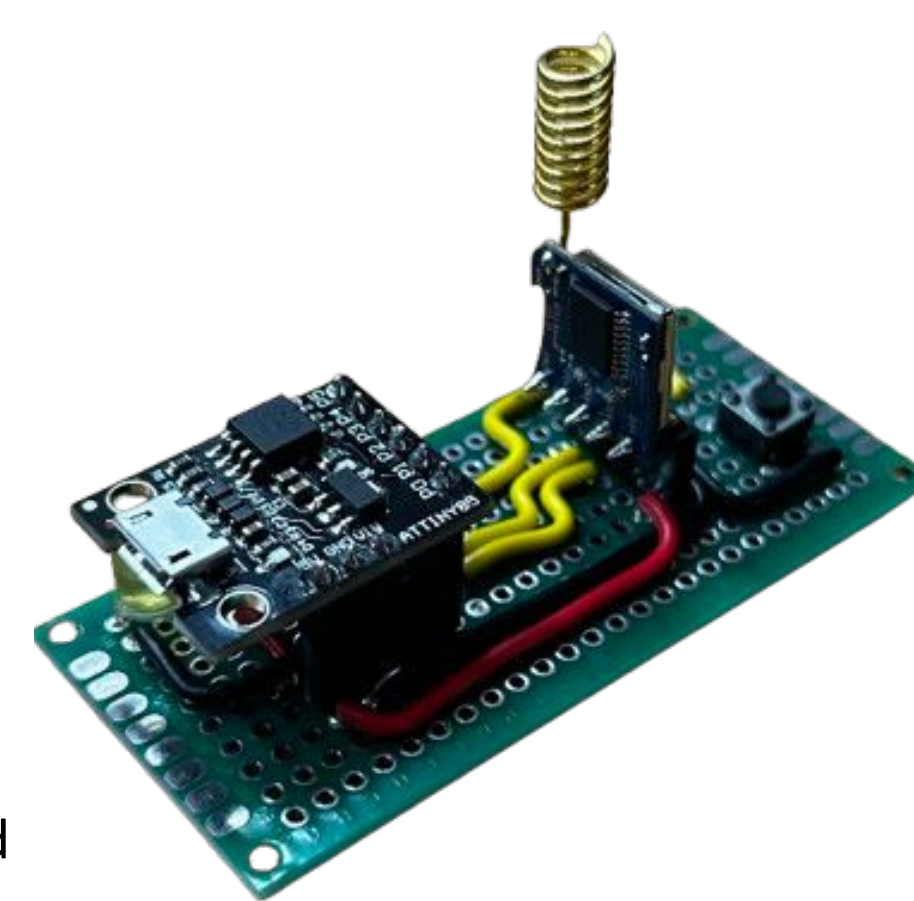
Fig 3 - current prototype of transmitter
